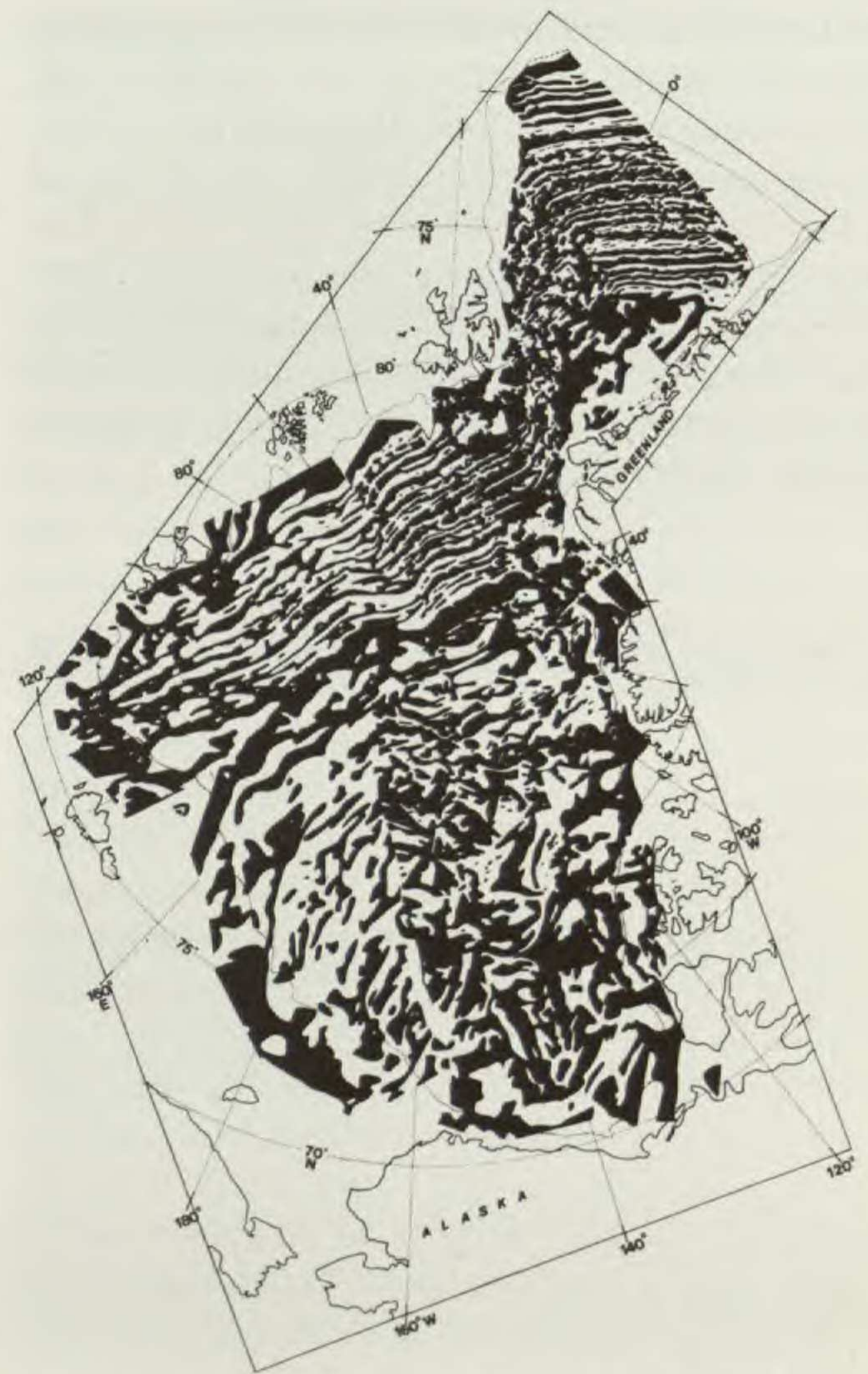
FIGURE 6. Magnetic anomalies of the Arctic Ocean and the northern Greenland-Norwegian Sea, showing medium-length anomalies greater than (black) and less than (white) the global magnetic reference field. The discontinuity near 160°W–60°E presents different data-reduction methods for the Soviet data, on the Eurasian side, and the generally more detailed U.S. Navy and Canadian data. Reproduced, with permission, from Vogt, Bernero, Kovacs and Taylor (1981, fig. 2).
